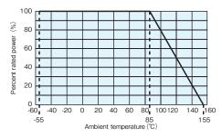
For resistors operated at an ambient temperature of 85°C or higher, the power shall be derated in accordance with the above derating curve.
